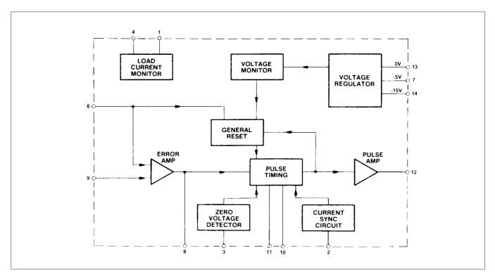
Fig. 2 Block Diagram of TDA2088
