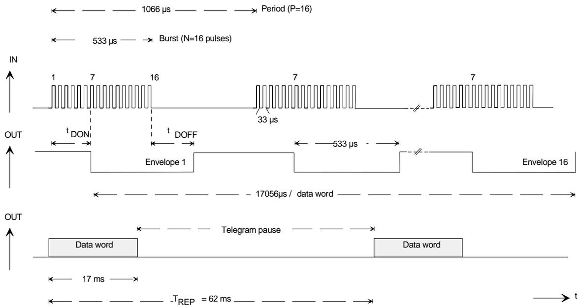
Example:  $f = 30 \text{ kHz}$ , burst with 16 pulses, 16 periods
