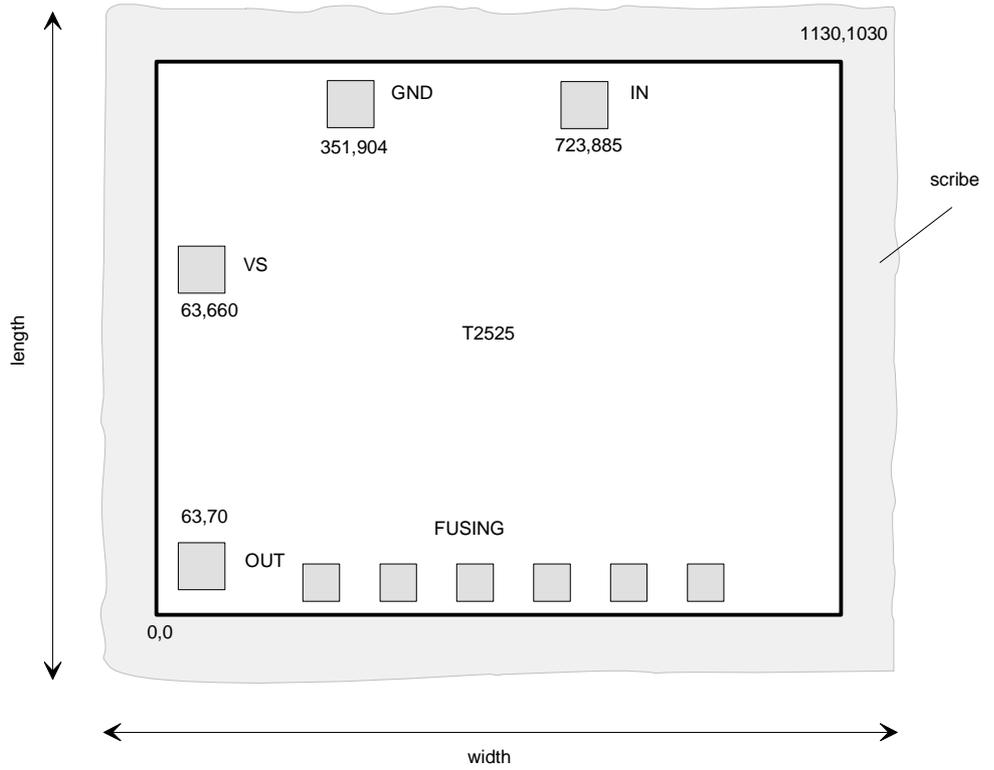
Note: Pad coordinates are for lower left corner of the pad in  $\mu\text{m}$  from the origin 0,0
