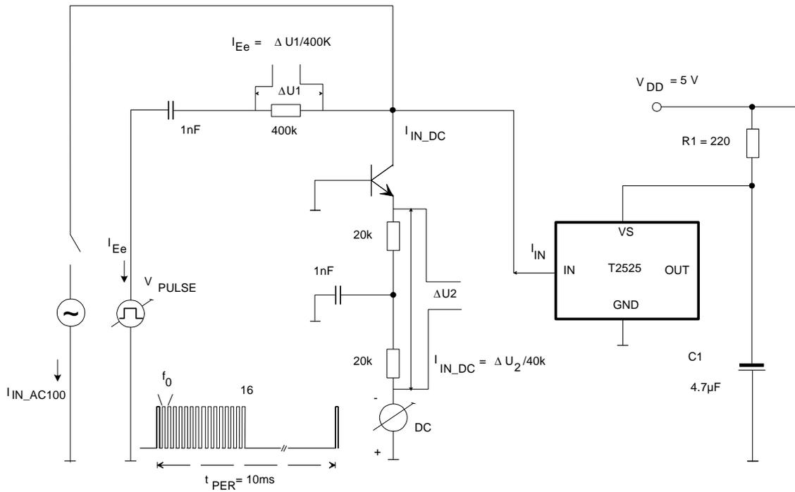
Figure 9. Application Circuit
