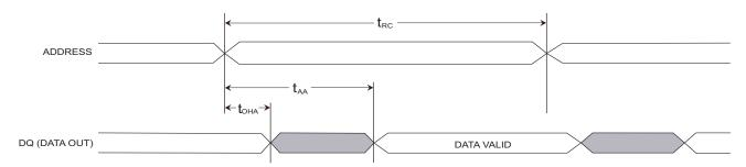
Figure 6. SRAM Read Cycle 2:  $\overline{\text{CE}}$  and  $\overline{\text{OE}}$  Controlled [5]
