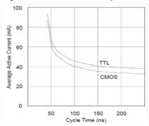
Figure 3. Current Versus Cycle Time (READ)
