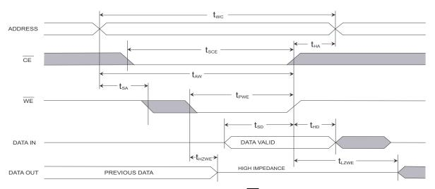
Figure 8. SRAM Write Cycle 2:  $\overline{\text{CE}}$  Controlled [8]
