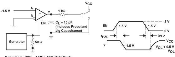
Generators: PRR = 1 MHz, 50% Duty Cycle,  $t_{r}$  <6 ns,  $\rm Z_{O}$  = 50  $\rm \Omega$
