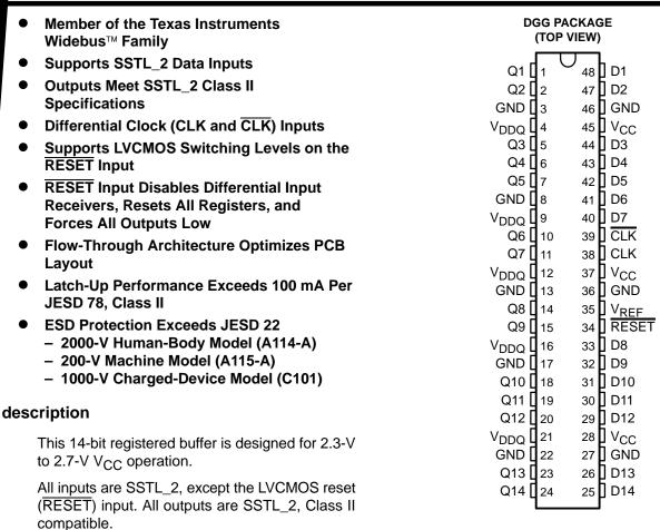
The SN74SSTV16857 operates from a differential clock (CLK and CLK). Data are registered at the crossing of CLK going high and CLK going low.
