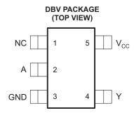
See mechanical drawings for dimensions. NC - No internal connection
