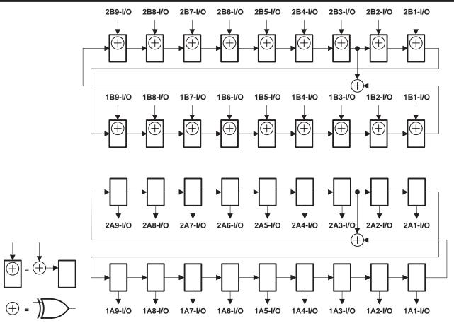
Figure 10. 18-Bit PSA/PRPG Configuration (1OEAB = 2OEAB = 1, 1OEBA = 2OEBA = 0)
