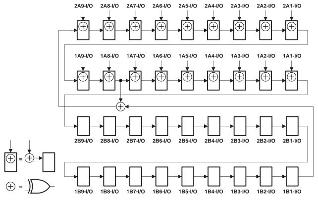
Figure 7. 36-Bit PSA Configuration (10EAB = 20EAB = 0, 10EBA = 20EBA = 1)
