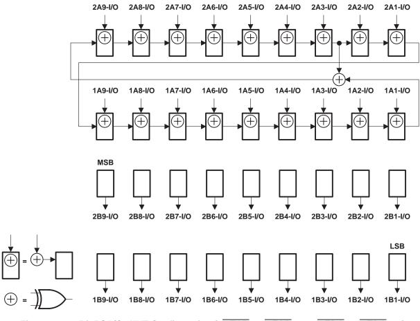
Figure 11. 18-Bit PSA/COUNT Configuration (10EAB = 20EAB = 0, 10EBA = 20EBA = 1)
