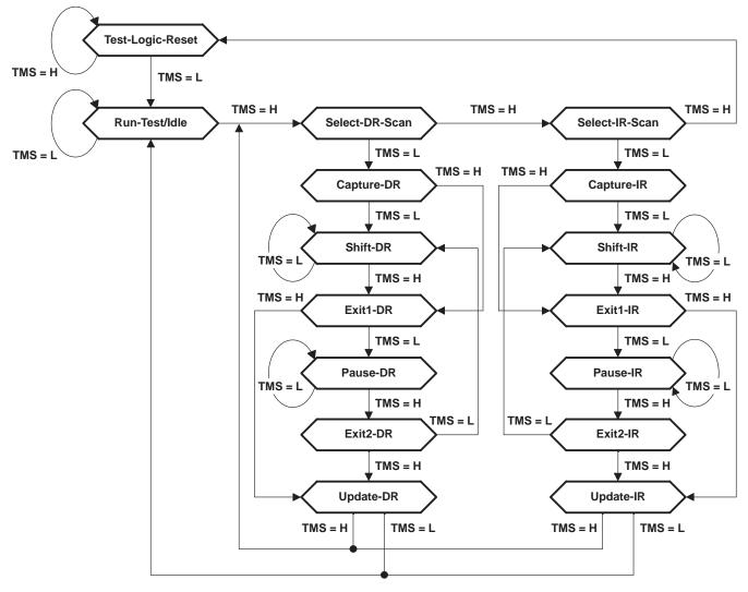
Figure 1. TAP-Controller State Diagram
