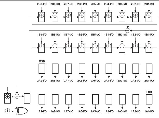
Figure 12. 18-Bit PSA/COUNT Configuration (1OEAB = 2OEAB = 1, 1OEBA = 2OEBA = 0)
