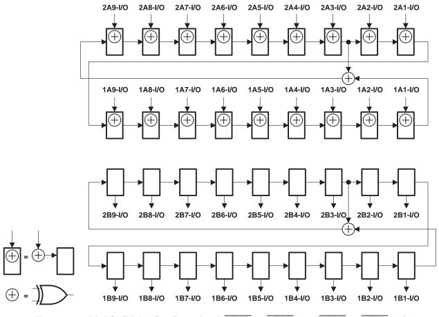
Figure 9. 18-Bit PSA/PRPG Configuration (10EAB = 20EAB = 0, 10EBA = 20EBA = 1)
