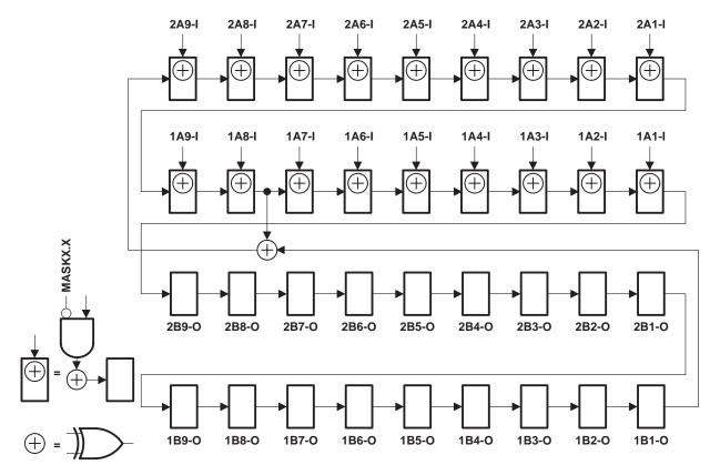
Figure 7. 36-Bit PSA Configuration (10EA = 20EA = 0, 10EB = 20EB = 1)
