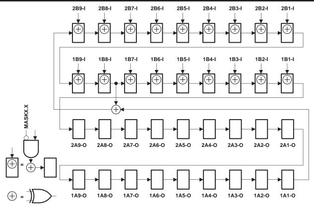
Figure 8. 36-Bit PSA Configuration (10EA = 20EA = 1, 10EB = 20EB = 0)
