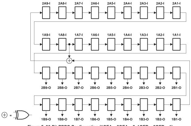
Figure 5. 36-Bit PRPG Configuration (10EA = 20EA = 0, 10EB = 20EB = 1)
