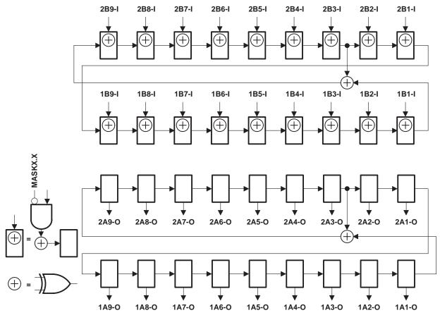
Figure 10. 18-Bit PSA/PRPG Configuration (10EA = 20EA = 1, 10EB = 20EB = 0)
