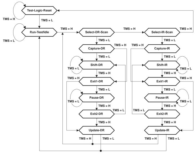
Figure 2. TAP-Controller State Diagram
