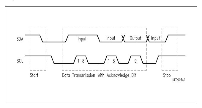
Figure 1 Operational States of the I<sup>2</sup>C Bus
