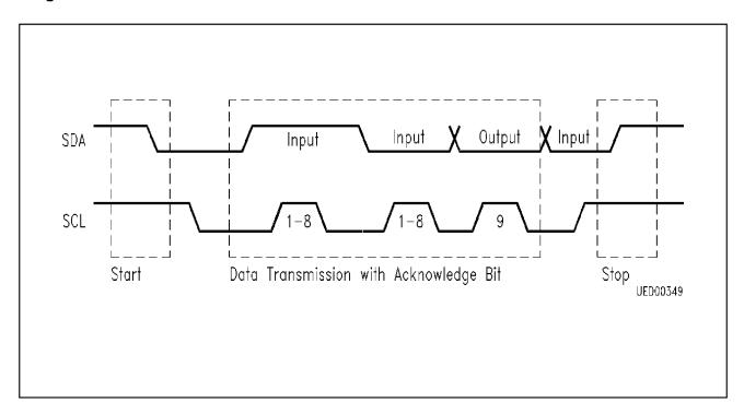
Figure 1 Operational States of the  $I^2C$  Bus
