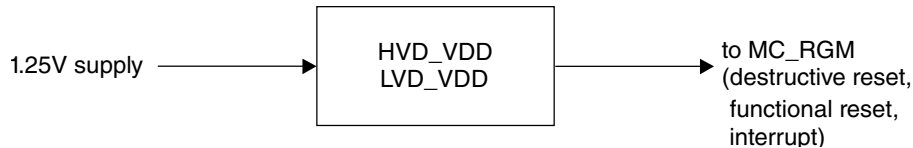
Figure 5-1. Logic scheme of the core voltage detectors
