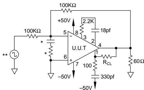
\* These components are used to stabilize device due to poor high frequency characteristics of burn in board.
