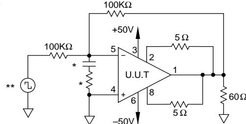
\* These components are used to stabilize device due to poor high frequency characteristics of burn in board.
