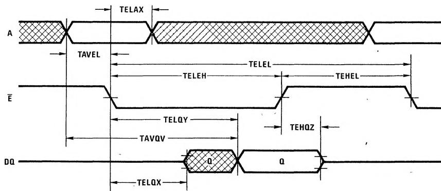
**Write Cycle AC Electrical Characteristics** over the operating range
