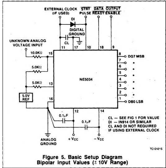
**Figure 5. Basic Setup Diagram
