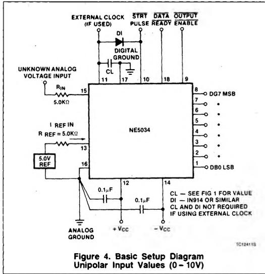
**Figure 4. Basic Setup Diagram
