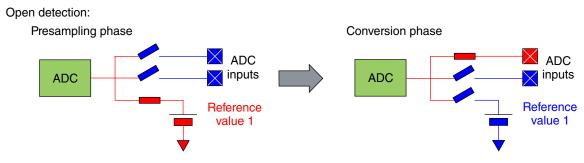
Figure 5-14. ADC\_SWTEST\_TEST1 (open detection)
