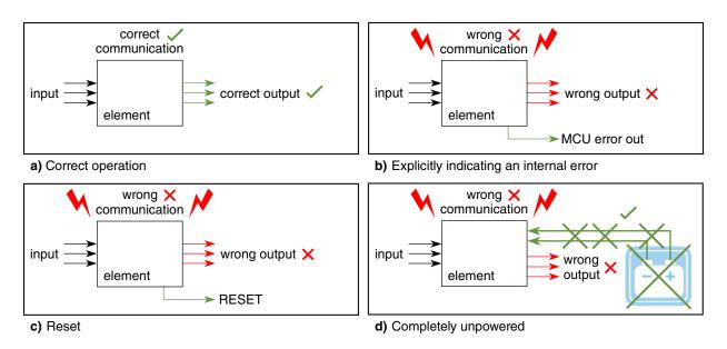
Figure 2-1. Safe state<sub>MCU</sub> of MPC5744P
