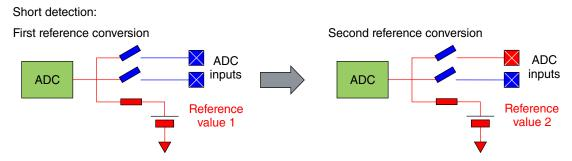
Figure 5-16. ADC\_SWTEST\_TEST2 (short detection)
