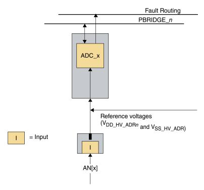
Figure 5-11. Single read analog input configuration
