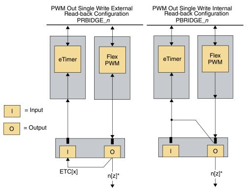
\*Note: n[z] represents any FlexPWM output (for example, A[z], B[z] or X[z]), but each output must be driven by different FlexPWM modules.
