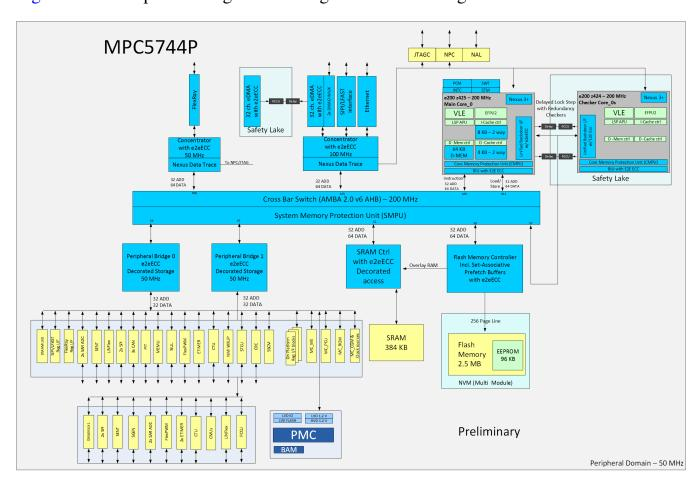
Figure 3-1. MPC5744P block diagram
