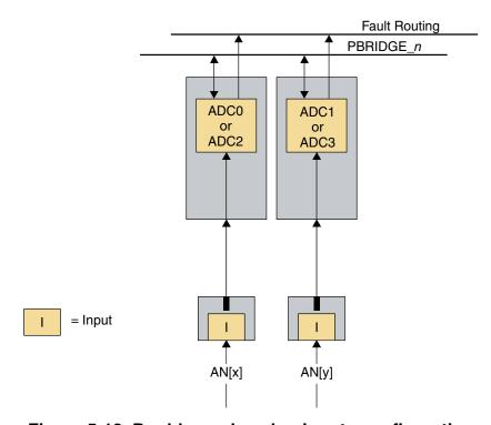
Figure 5-12. Double read analog inputs configuration
