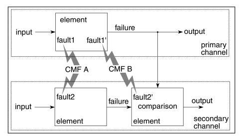
Figure 2-4. Common Mode failures
