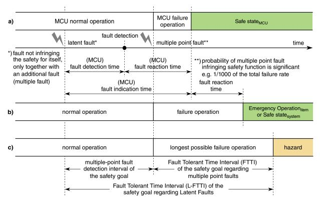
Figure 2-7. Fault Tolerant Time Interval for latent faults
