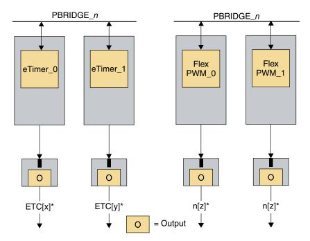
Note: n[z] represents any FlexPWM output (for example, A[z], B[z] or X[z]), but each output must be driven by different FlexPWM modules. The same consideration is valid for the eTimer; any eTimer output may be used, but each output must be driven by different eTimer module.
