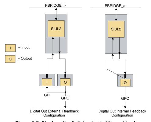
Figure 5-7. Single write digital output with read-back
