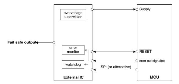
Figure 4-1. Functional safety related connection to external circuitry
