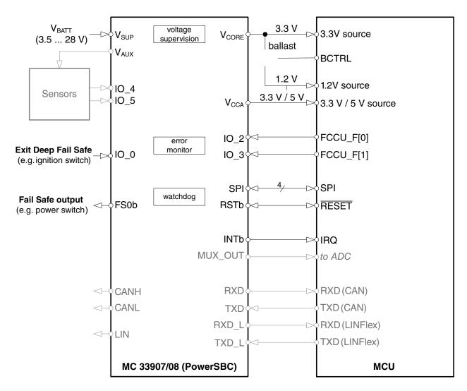
Figure 4-2. Functional safety application with PowerSBC
