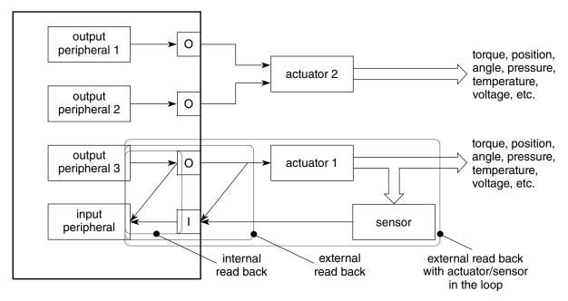
Figure 5-6. Digital Outputs with redundancy and read back
