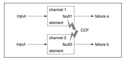
Figure 2-3. Common Cause Failures
