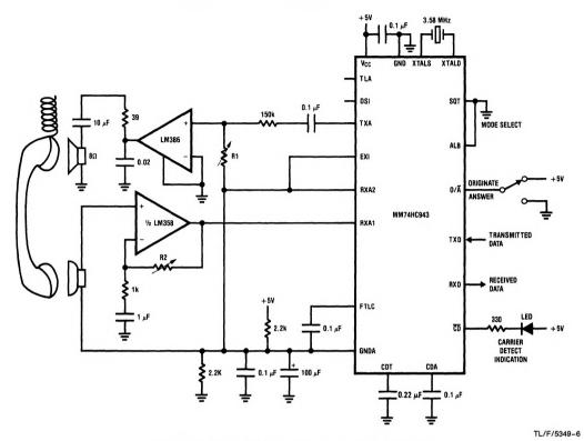
Note: The efficiency of the acoustic coupling will set the values of R1 and R2.
