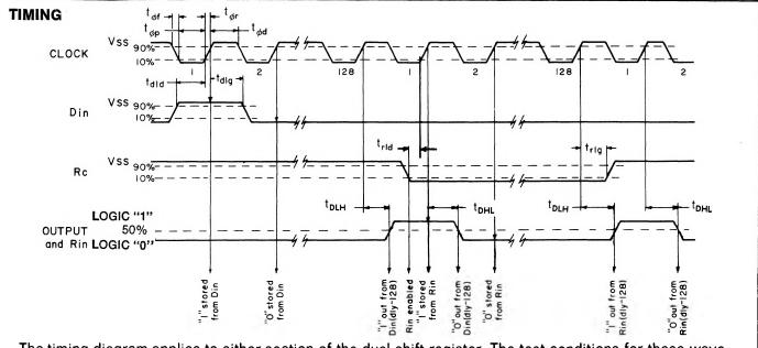
The timing diagram applies to either section of the dual shift register. The test conditions for these waveforms are illustrated below. A logic "1" is defined as +5 V and a logic "0" is defined as OV
