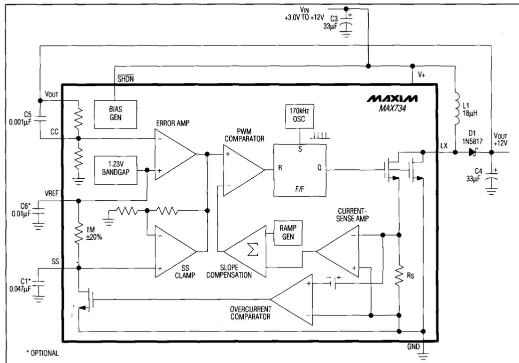
Figure 2. Detailed Block Diagram with External Components
