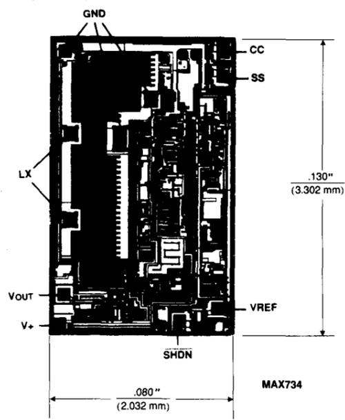
NOTE: SUBSTRATE CONNECTED TO V+;
