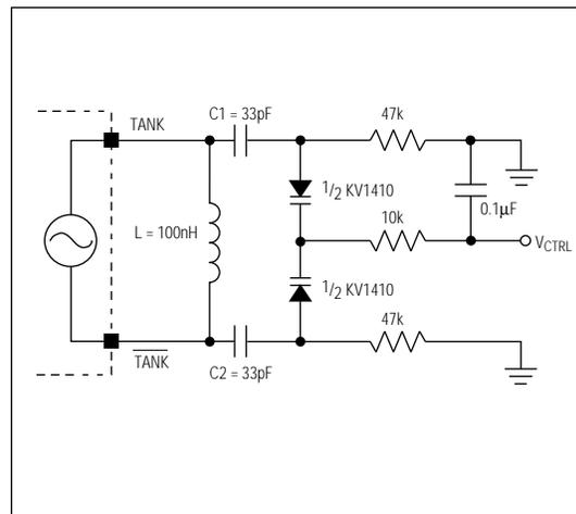
Figure 4. Typical Resonant Tank Circuit
