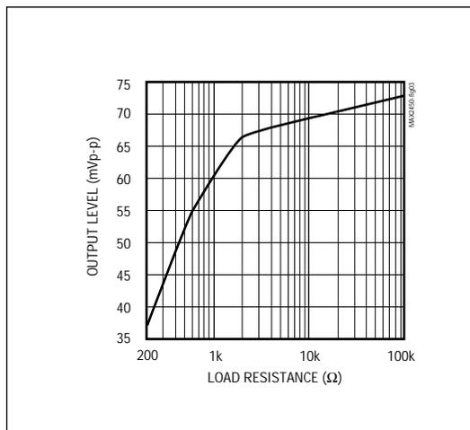
Figure 3. Modulator Output Level vs. Load Resistance
