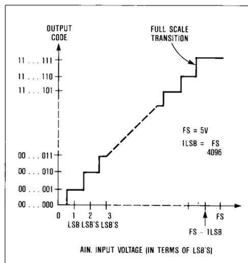
Figure 14. MAX163 Unipolar Transfer Function
