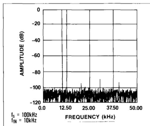
Figure 18. FFT Plot for the MAX167
