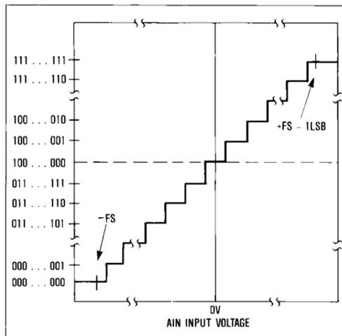
Figure 15. MAX164/167 Bipolar Transfer Function
