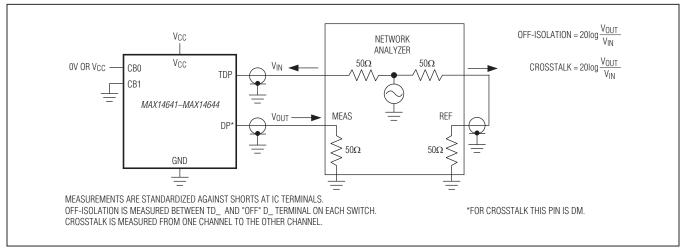
Figure 3. Bandwidth, Off-Isolation, and Crosstalk
