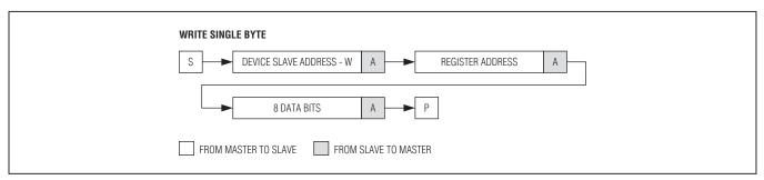
Figure 8. Write Byte Sequence
