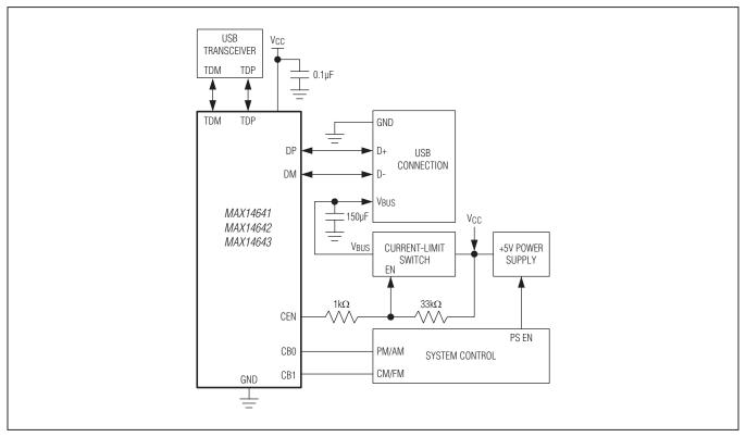
Figure 6. MAX14641/MAX14642/MAX14643 Peripheral Reset Applications
