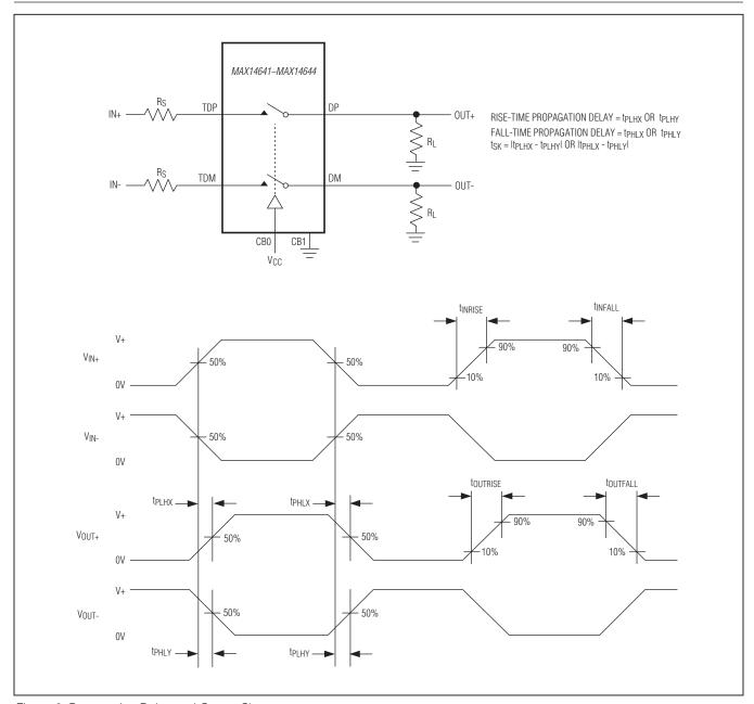
Figure 2. Propagation Delay and Output Skew
