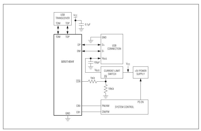
Figure 5. MAX14644 Peripheral Reset Applications Diagram
