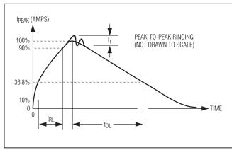
Figure 14. Human Body Current Waveform
