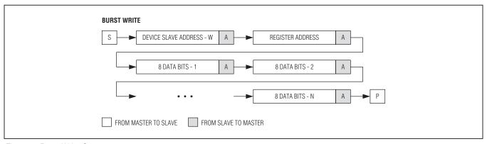
Figure 9. Burst Write Sequence
