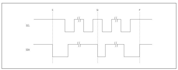
Figure 7. I<sup>2</sup>C START, STOP, and Repeated START Conditions
