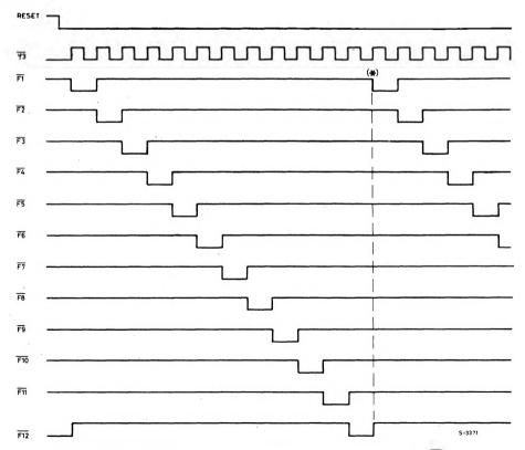
Note: The matrix scanning starts (after the power on reset) at the second arrival in output of F1 (\*) from B1 to B6 in continuous sequence.
