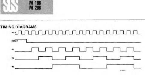
Note: MCK is the master clock input (matrix scanning),  $\varphi 1$ ,  $\varphi 2$ ,  $\varphi 3$  are internal phases to generate  $F1 \div F12$ .
