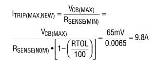
Since  $I_{TRIP(MAX, NEW)} > I_{LOAD(MAX)}$ , a larger value for  $R_{SENSE}$  should be selected and the process repeated again to lower  $I_{TRIP(MAX, NEW)}$  without substantially affecting  $I_{LOAD(MAX)}$ .
