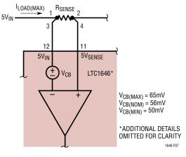
Figure 7. Circuit Breaker Equivalent Circuit for Calculating R<sub>SENSE</sub>
