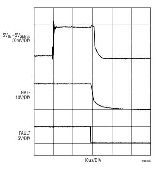
Figure 5. Overcurrent Fault on 5V
