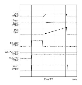
Figure 4. Power-Up into a Short on 3.3V Output
