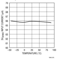
3V<sub>IN</sub> Input Current vs Temperature
