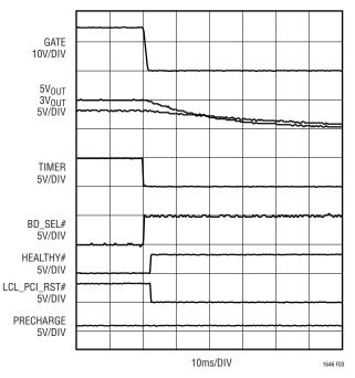
Figure 3. Normal Power-Down Sequence
