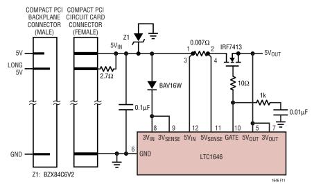
Figure 11. 5V Supply Only Typical Application
