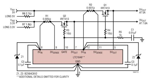
Figure 13. Place Transient Protection Device Close to the LTC1646
