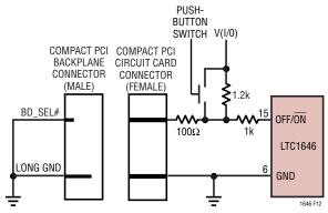
Figure 12. BD\_SEL# Pushbutton Toggle Switch
