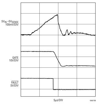
Figure 6. Short-Circuit Fault on 5V
