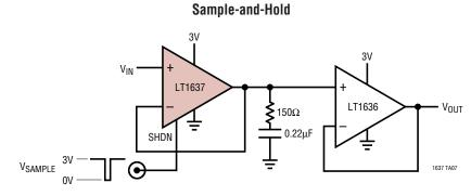
DROOP (LT1636 BUFFER): 200mV/s DROOP INTO HIGH IMPEDANCE : LESS THAN 0.625mV/s
