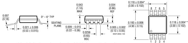
\* DIMENSION DOES NOT INCLUDE MOLD FLASH, PROTRUSIONS OR GATE BURRS. MOLD FLASH, PROTRUSIONS OR GATE BURRS SHALL NOT EXCEED 0.006" (0.152mm) PER SIDE
