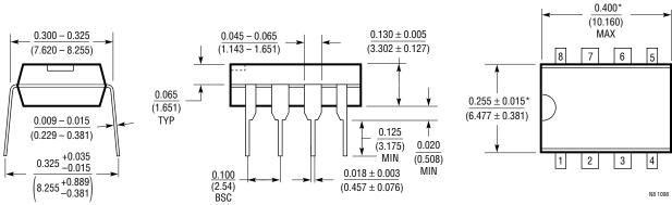
\*THESE DIMENSIONS DO NOT INCLUDE MOLD FLASH OR PROTRUSIONS. MOLD FLASH OR PROTRUSIONS SHALL NOT EXCEED 0.010 INCH (0.254mm)
