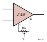
Figure 1. Input Offset Nulling
