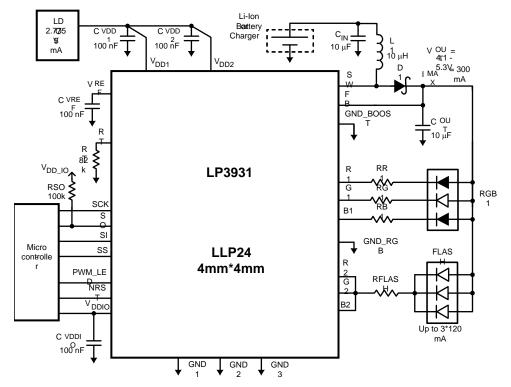
Figure 21. LP3931 with One RGB and One FLASH LED
