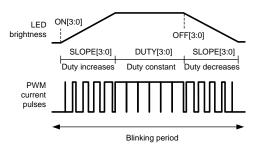
Figure 18. RGB PWM Operating Principle
