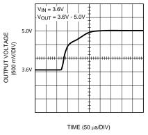
Figure 15. Boost Startup with No Load
