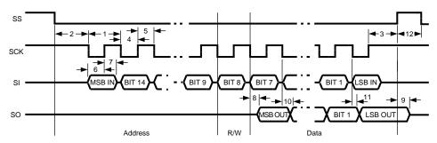
Figure 7. SPI Timing Diagram
