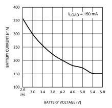
Figure 12. Battery Current vs Voltage
