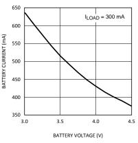
Figure 13. Battery Current vs Voltage
