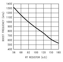
Figure 11. Boost Frequency vs RT Resistor
