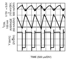
Figure 14. Boost Typical Waveforms at 100 mA Load
