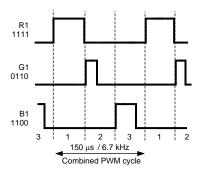
Figure 19. Normal Mode PWM Waveforms at Different Duty Settings
