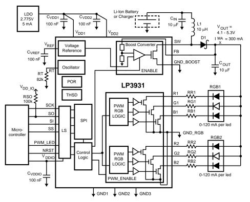
Figure 4. LP3931 Block Diagram
