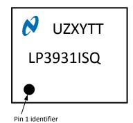
Figure 3. Package Mark—Top View
