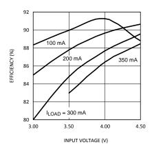
Figure 10. Boost Converter Efficiency
