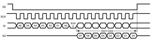
Figure 6. SPI Read Cycle
