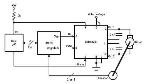
Figure 14. Basic Motor Driver
