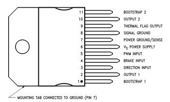
Figure 2. Top View See Package Number NDJ0011B
