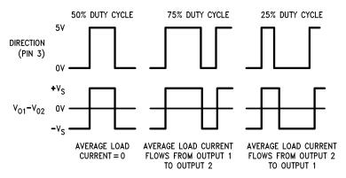
Figure 9. Locked Anti-Phase PWM Control
