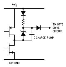
Figure 12. Internal Charge Pump Circuitry
