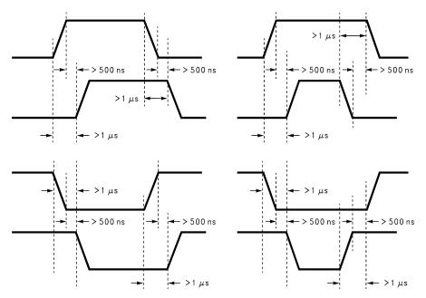
Figure 11. Transitions in Brake, Direction, or PWM Must be Separated by At Least 1 µsec
