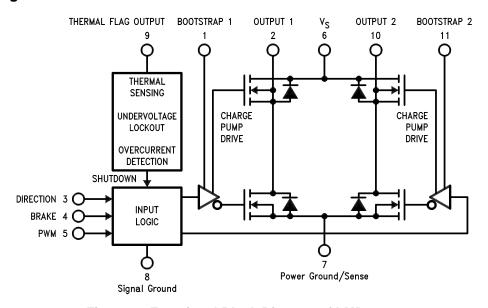
Figure 1. Functional Block Diagram of LMD18201
