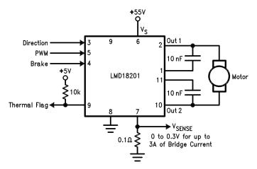
Figure 15. Current Sensing
