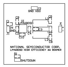
Figure 2. Recommended SD PCB Layout Top Silkscreen
