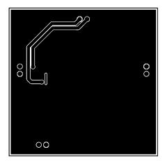
Figure 4. Recommended SD PCB Layout Bottom Layer
