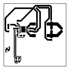
Figure 3. Recommended SD PCB Layout Top Layer
