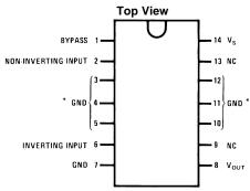
Figure 3. Dual-In-Line Package
