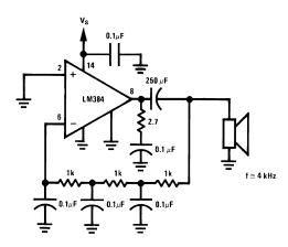
Figure 7. Phase Shift Oscillator
