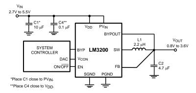
Figure 33. Typical Operating System Circuit
