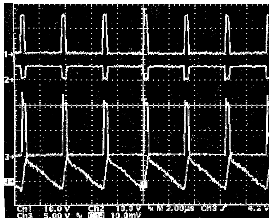
Figure 6. Normal FPWM Mode Operation at Light Loads
