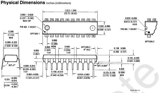
Molded Dual-In-Line Package (N) Order Number LM1818N NS Package Number N20A
