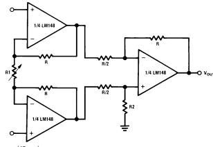
$V_{OUT} = 2 \bigg( \frac{2R}{R1} + 1 \bigg) \text{ , } V_{\overline{S}} - 3V \leq V_{IN \text{ CM}} \leq {V_{\overline{S}}}^+ - 3V,$
