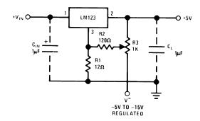
Figure 15. Trimming Output to 5V
