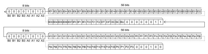
Note : After the above serial data is sent, the contents of the display data can be changed by transferring only the serial data (CCB address, display data, fixed data, and direction data) including the display data to be changed in 64-bit units.
