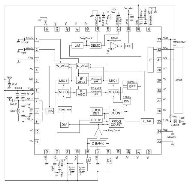
\* Culprits oscillation circuit is used in this IC as a crystal oscillation circuit. Caution is required for layout of the board because oscillation between pin25 and power source and GND line.
