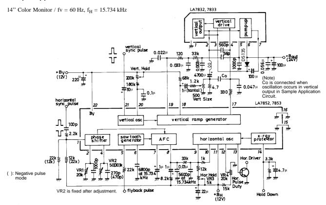
(Note) For the LA7853, the vertical pull-in range is 20 Hz at vertical sync 60 Hz.
