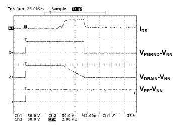
Figure 8 - Turn on Waveforms
