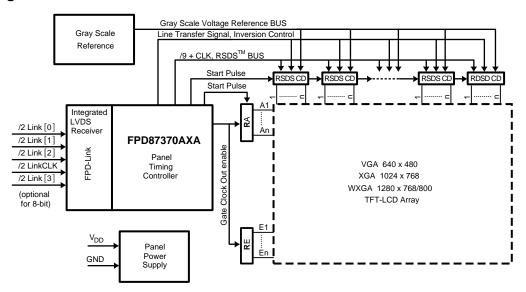
Figure 1. Block Diagram of the LCD Module
