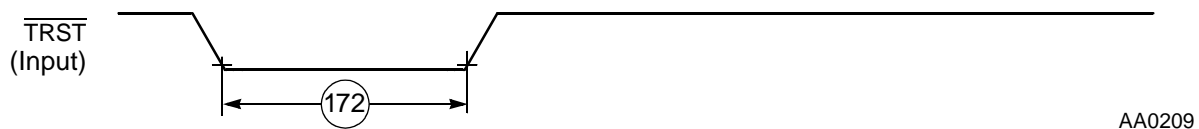
Figure 36. \overline{\text{TRST}} Timing Diagram
