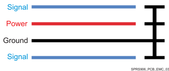
Figure 8-13. Guard Ring Routing
