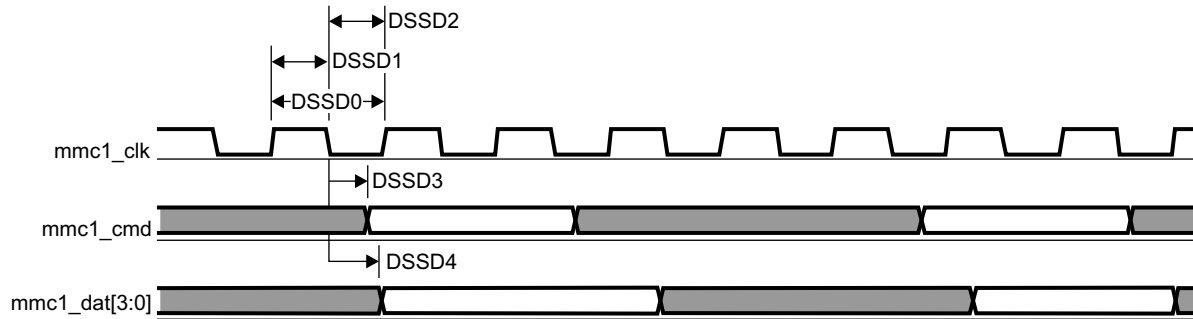
Figure 7-63. MMC/SD/SDIO in - Default Speed - Transmitter Mode
