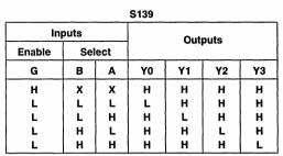
H = high level, L = low level, X = don't care (either low or high logic level)
