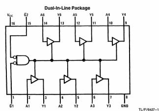
Order Number 54LS365ADMQB, 54LS365AFMQB, 54LS365ALMQB, DM54LS365AJ, DM54LS365AW, DM74LS265AM or DM74LS365AN See NS Package Number E20A, J16A, M16A, N16E or W16A
