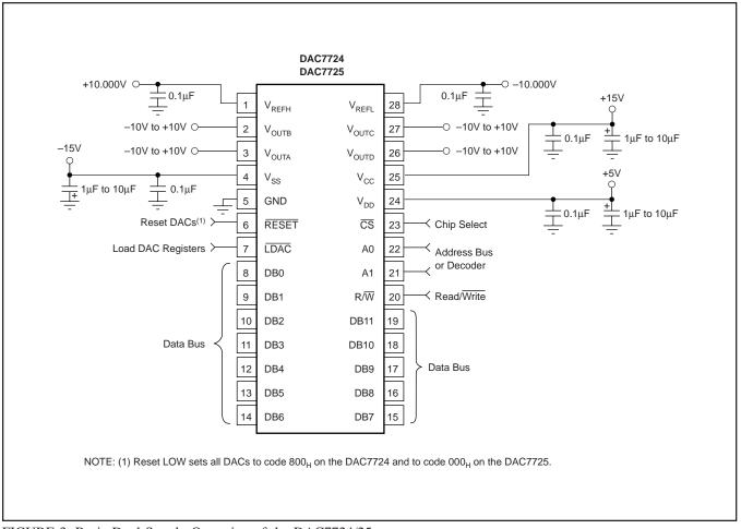
FIGURE 3. Basic Dual-Supply Operation of the DAC7724/25.
