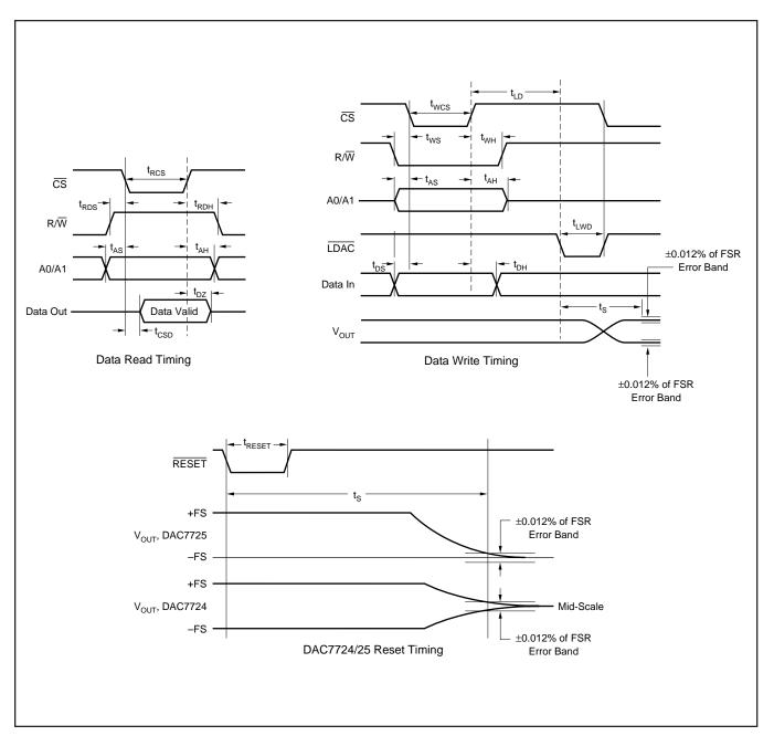
FIGURE 4. Digital Input and Output Timing.
