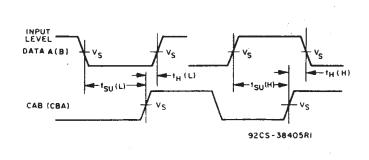
Fig. 4 - Data setup and hold times.
