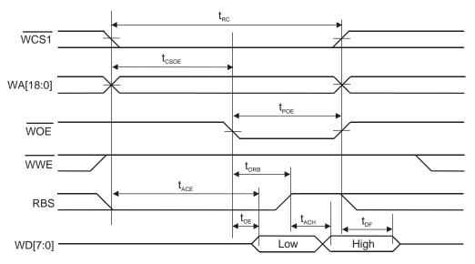
Figure 7. 8-bit SRAM Write Cycle
