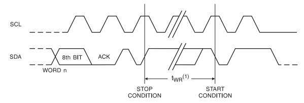
Note: 1. The write cycle time t<sub>WR</sub> is the time from a valid stop condition of a write sequence to the end of the internal clear/write cycle.
