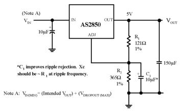
Fig. 6 Improving Ripple Rejection
