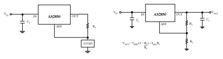
Fig. 4 5A Current output Regulator
