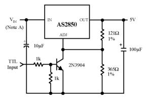
Note A:  $V_{IN(MIN)}$  = (Intended  $V_{OUT}$ ) + ( $V_{DROPOUT (MAX)}$ )
