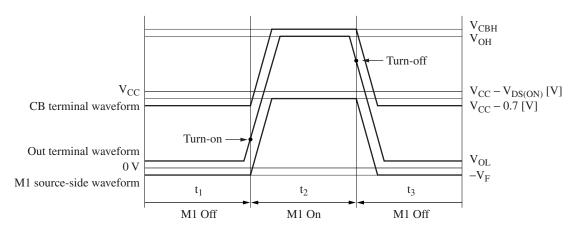
Figure 7. Bootstrap circuit operation waveform
