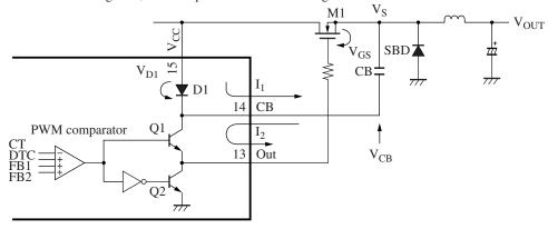
Figure 6. Output block and bootstrap circuit
