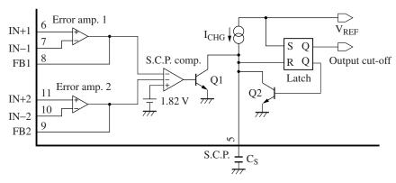
Figure 4. Short-circuit protection circuit
