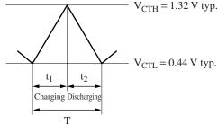
Figure 1. Triangular wave oscillation waveform
