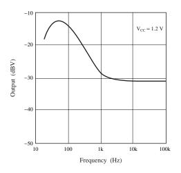
Distortion and amplitude characteristics of headphone amp. Input — Distortion/output voltage
