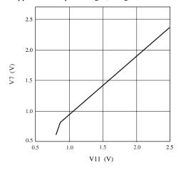
10. Pin 2 (V<sub>REF</sub>) at standby on/off and voltage at pin 7 (Ripple filter)
